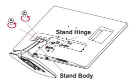
4 1 Turn the screw to the left.2 Pull out the Stand Base.
